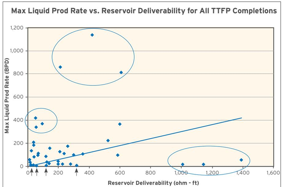
Figure 4 – Maximum liquid production rate (oil + water) vs. reservoir deliverability for all TTFP completions in western GOM
