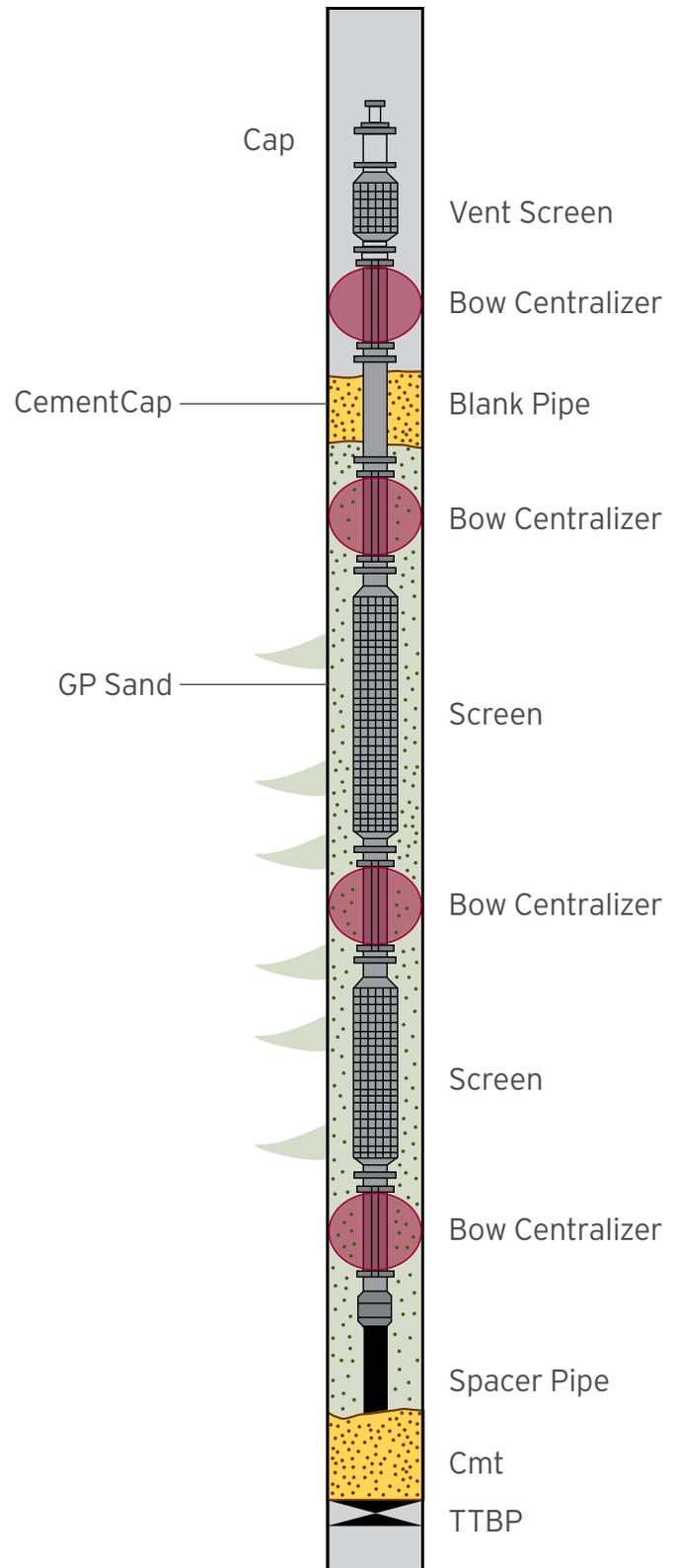
Figure 2 – Typical Thru-Tubing Gravel Pack assembly
