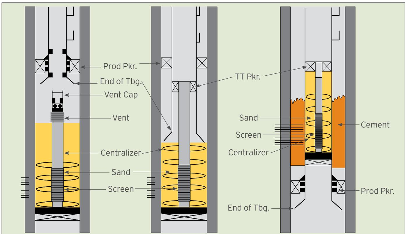
Figure 3 – (Left) “Vent Screen,” or “Non-packer” TTFP assembly, (center) “Packer” TTFP assembly, (right) “Cement Packer” TTFP assembly
