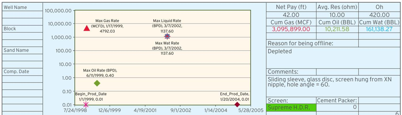
Figure 5 – “Well Card” shows basic production history data for each completion in the database
