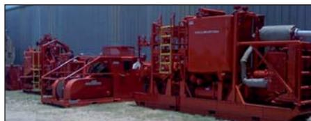
*The deck spread includes a double-drum slickline and e-line unit, the cement unit, a cement lab, P-tanks, dual circulating pump skids and complete gas buster and flow-back package. Pictured are the dual circulation pumps, the double-drum slickline/e-line unit and the cement unit.*
