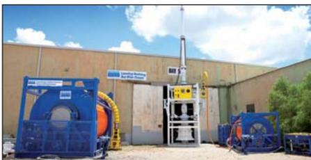
*The subsea spread consists of the BOP stack, the hydraulic and circulation umbilicals, the disconnect capability and tooling. Pictured are the umbilicals and the lubricator.*
